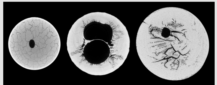
Figure 25. Microgravity samples show fractured structures upon crystallization. Images provided by the ELF research team.
