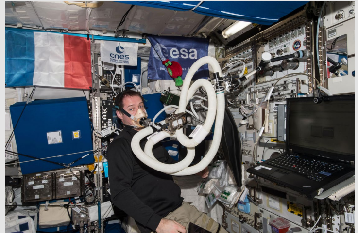
Figure 17. ESA astronaut Thomas Pesquet in the Columbus Module using the Pulmonary Function System to perform a series of oxygen uptake measurements after prescribed meals and scheduled fluid collections. NASA ID: iss050e055526.
